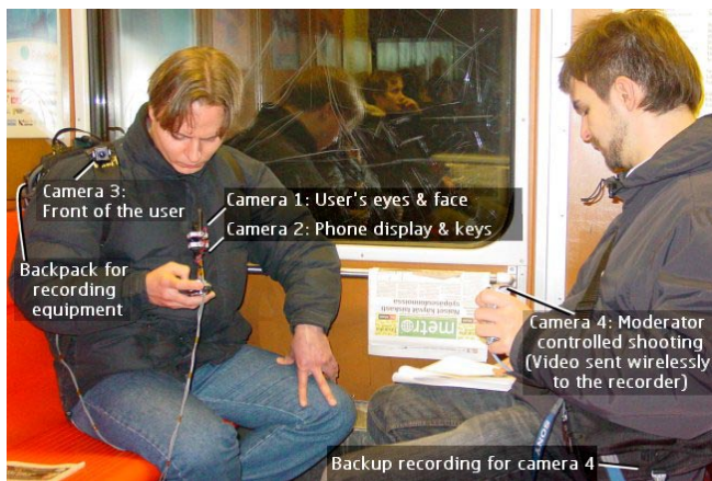
Figure 4. Configuration of recording equipment.
