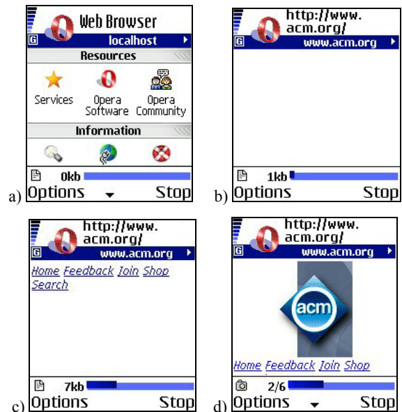
Figure 2. Opera browser user interface changes during the four download phases of Figure 1.
