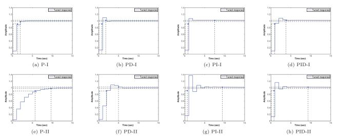
Figure 6: Step response (MovieLens 1m). The first point represents the rise time of the system (90% of the target value) and the second point marks when the system reaches steady state. The first row shows the fast controllers with 2-5 sec response time, and the second row has the slower controllers with 5-10 sec response time.
