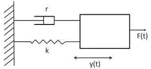
Figure 3: A mass attached to a spring and damper. y(t) is the displacement. The damping coefficient is represented by r in this case, where the spring constant is k. F(t) in the diagram denotes an external force. In our case, y(t) is the performance value while F(t) = u(t) number of new training samples.
