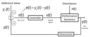
Figure 4: The time domain block diagram.
