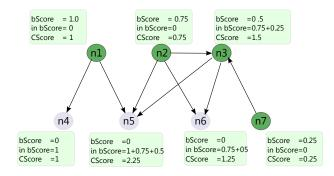
Figure 1: Example of  $S_C$  computation for a simple graph. Parameter k = 4, the nodes n1,n2,n3,n7 (in this order) are the top k matches for document similarity to the query.
