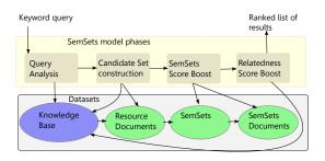
Figure 2: Block scheme of the SemSets model computation process. The upper block describes of model phases, while the lower block represents the data sets used in distinct phases.
