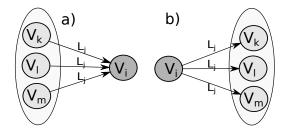
Figure 3: SemSets patterns in a property graph structure. A SemSet is a) vertices having outgoing edge of the same label to a common vertex, b) vertices having an incoming edge of the same type from a single vertex.
