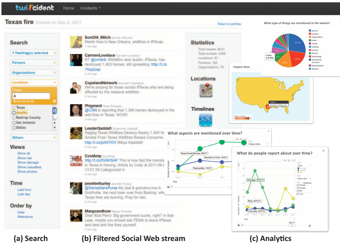
Figure 3: Screenshot of the Twitcident system: (a) search and filtering functionality to explore and retrieve particular Twitter messages, (b) messages that are related to the given incident (here: fires in Texas) and match the given query of the user and (c) realtime analytics of the matching messages.
